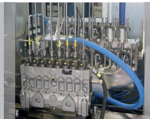
Inline pump setup
