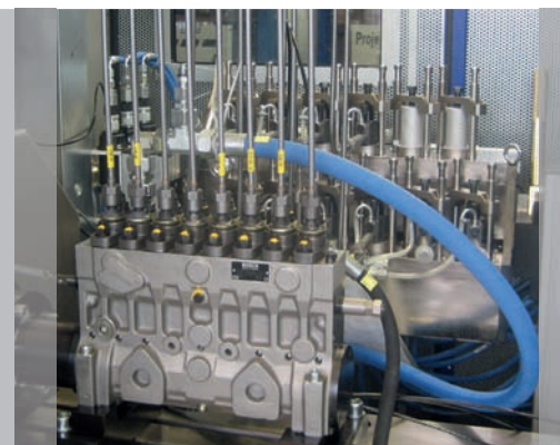
Inline pump setup
